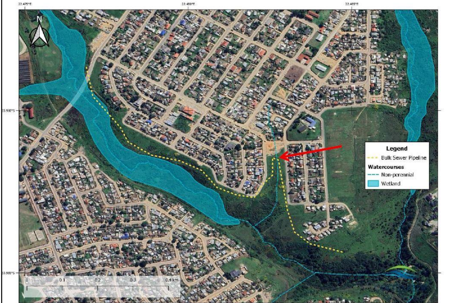
APPENDIX B2: FIGURE 2: MAP SHOWING THE DELINEATED EXTENT OF SEEP WETLANDS ALONG THE MEUL RIVER AND ITS EASTERN TRIBUTARY. THE PIPELINE CROSSES A STORMWATER CHANNEL AT THE POSITION INDICATED BY THE RED ARROW.
