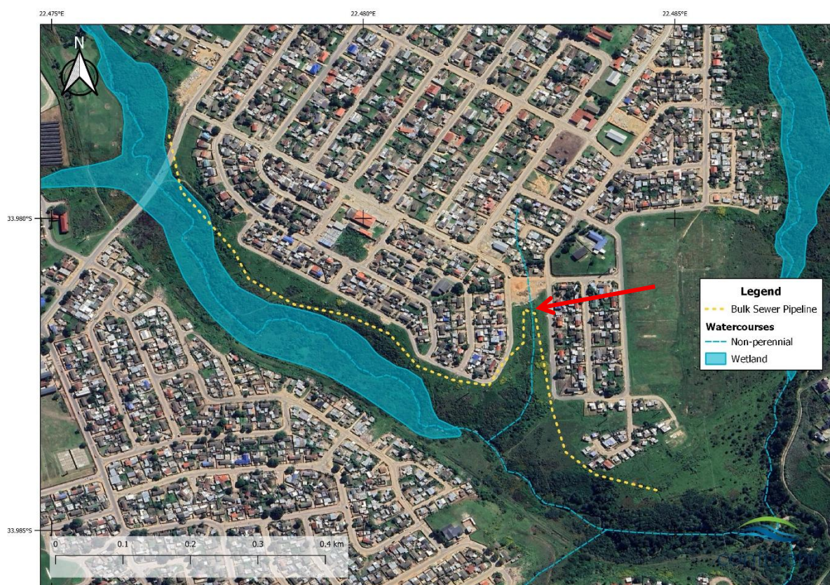
Figure 10: Map showing the delineated extent of seep wetlands along the Meul River and its eastern tributary. The pipeline crosses a stormwater channel at the position indicated by the red arrow.
