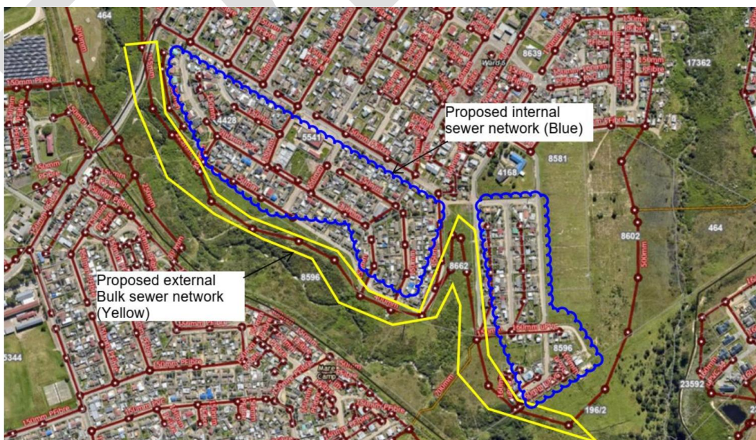
Figure 4: Proposed Sewer Scope of Work
