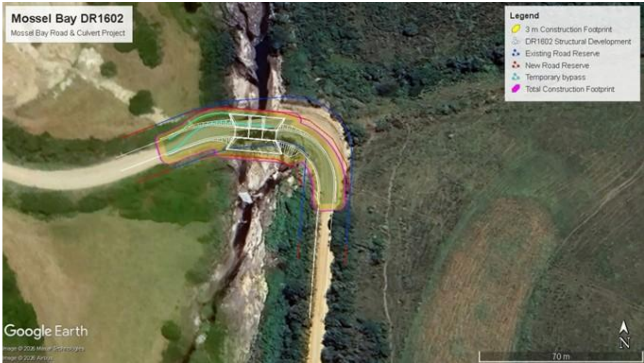
Figure 2. The Proposed Construction for Dr1602 Mossel Bay with a new road reserve, positioned slightly south.
