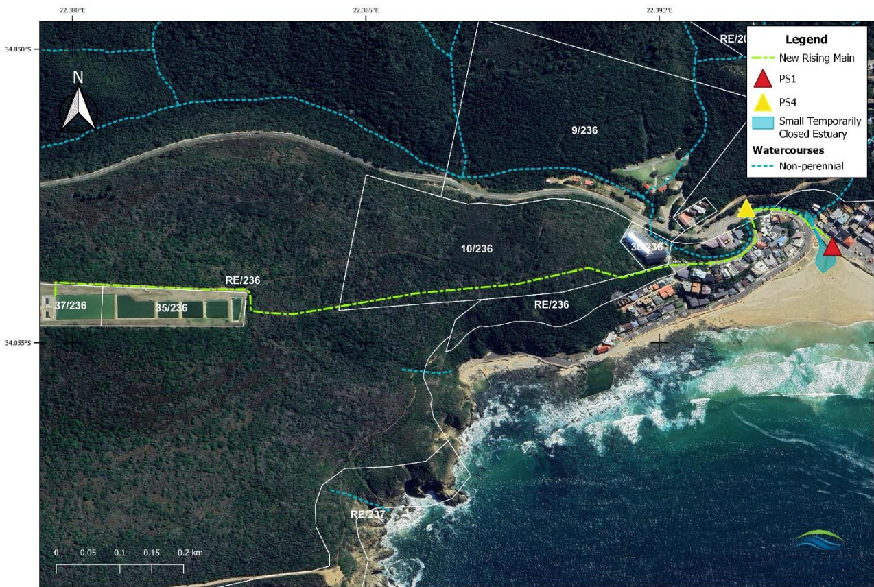
Figure 5: Map showing the alignment of the new rising main from PS1 to PS4 and from PS4 to the WWTW.
