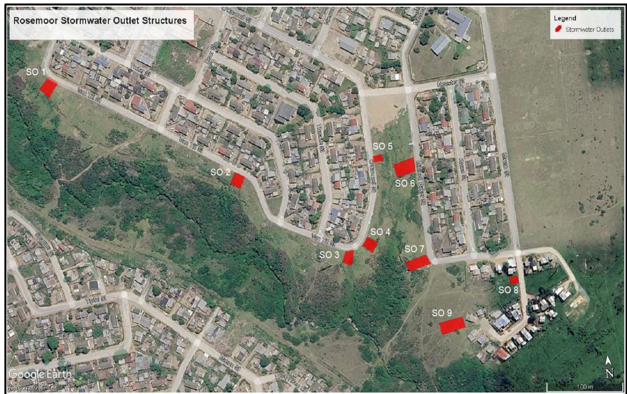
Figure 20: Proposed Stormwater Outlet Structures.
