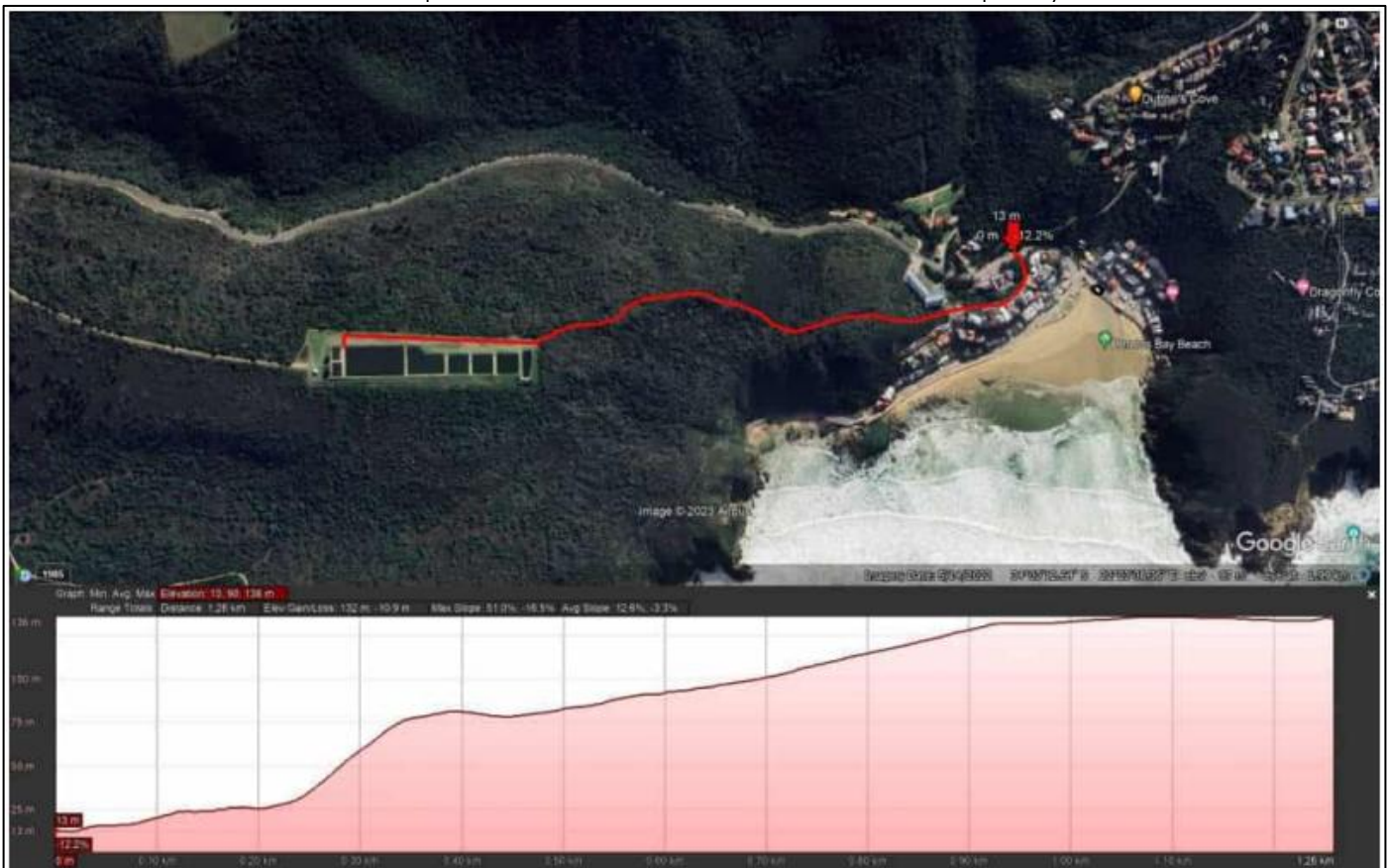
Figure 3: Pipeline route and vertical profiles for the pipeline between PS4 to WWTW
