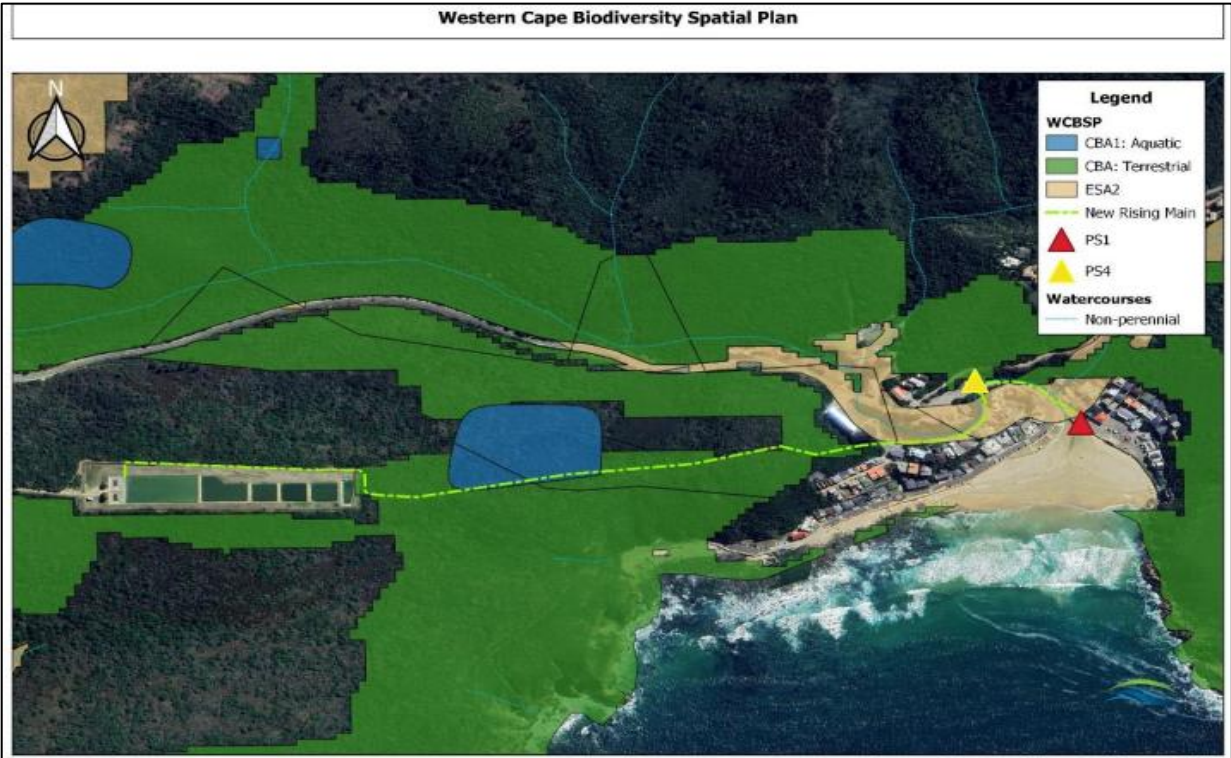
Figure 18: Map of the rising main alignment in relation to the Western Cape Biodiversity Spatial Plan (WCBSBP).
