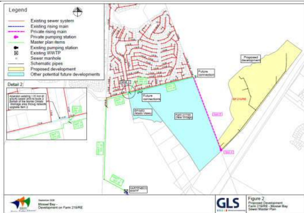
Figure 1. Proposed external sewer line.
