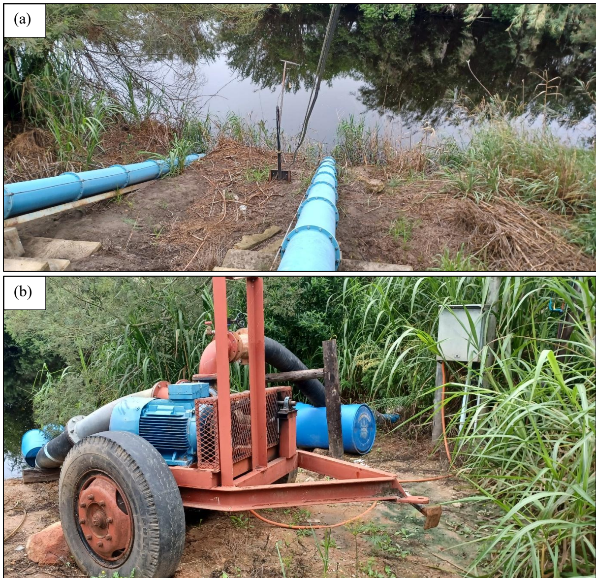
Plate 5: The abstraction point of the pumpstation (a), (b) one of the farmer's three large pumps abstracting water from the weir
