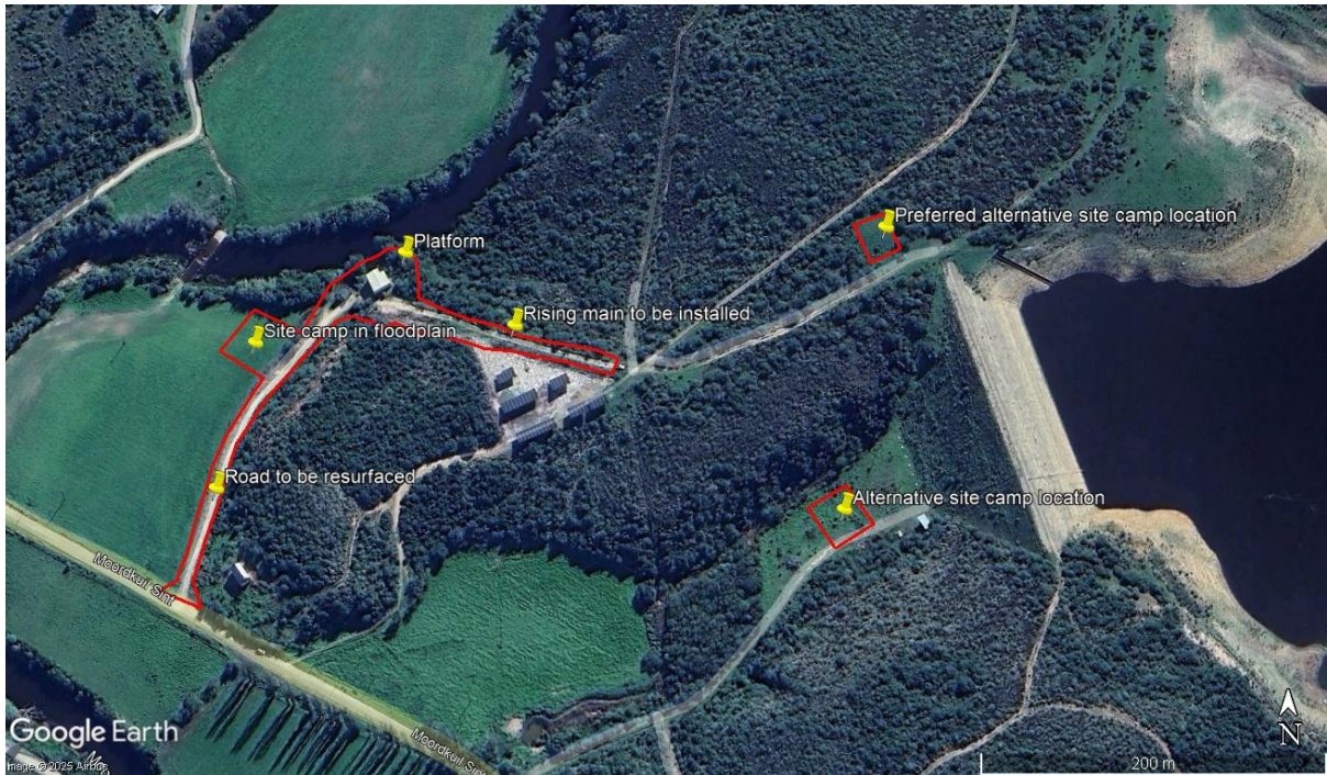
Figure 1: Google Earth site map for the Moordkuil River pump station upgrade and two sites for the proposed camp site.
