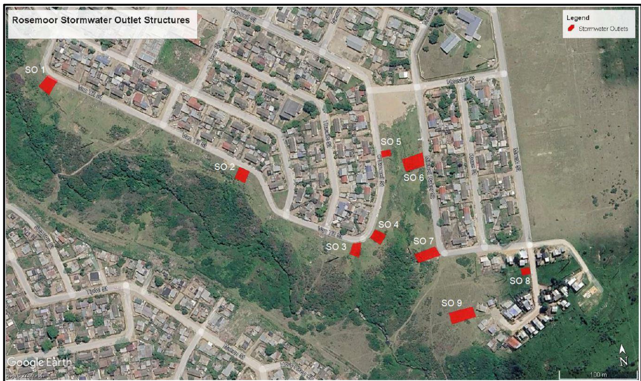
Figure 6: Proposed stormwater outlet structures.
