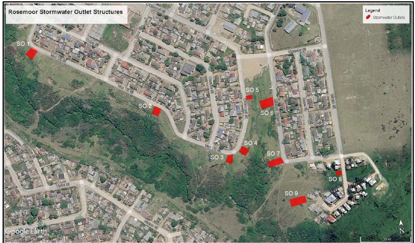
Figure 12: Proposed Stormwater Outlet Structures.
